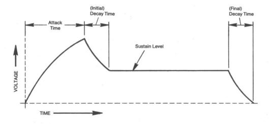
Each envelope comprises four parts: the initial rise time or attack—set by the ATTACK knob; the initial decay time or subsiding from maximum to the sustain level—set by the DECAY knob; the level at which the tone may be held indefinitely by holding a key down—set by the SUSTAIN knob; and the final release time which determines the time it takes the tone to fall to silence—set by the RELEASE knob.
