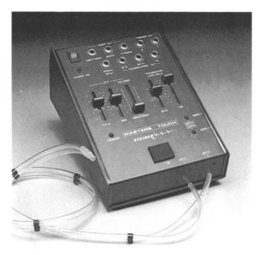
The MASTER'S TOUCH has a VCF and VCA that can act in lieu of those within the STRAUS (or other keyboard). When a special breath tube is blown, any signal passing through the MASTER'S TOUCH will be articulated (and filtered). Your breath acts like an envelope generator that is varied as you blow; the signal produced by blowing the breath tube controls the cutoff/gain of the VCF and VCA in the MASTER's TOUCH.
