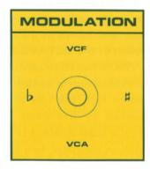
To the left of the keyboard is a joystick that lets you introduce several effects during performance. This is an "X-Y" joystick capable of movement in two planes (directions X and Y). Lateral movement of the joystick, in the
