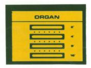
The sliders in the ORGAN section govern the loudnesses of the various footages" that are analogous to pipe organ pipe lengths. The ORGAN sliders increase loudness as they are moved to the right. They work in conjunction with the ORGAN VOLUME knob; that is, both must be set properly to provide output at either the POLYSYNTH or ORGAN output jack on the rear of the STRATUS. Turn the ORGAN VOLUME knob to 10 and experiment with different mixes of the 16', 8', 4', and 2' ORGAN sliders.
