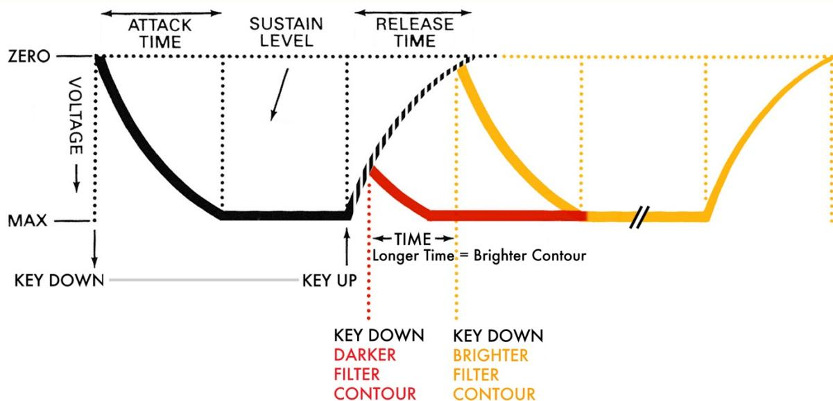
As the inverted FILTER CONTOUR slowly *rises*—rather than *falls*, if a *later* KEY DOWN occurs, a new ATTACK TIME will be started. As the graphic shows, a *later* KEY DOWN time will catch the RELEASE TIME at a *later* time on its upward trajectory, and a brighter ATTACK TIME will occur. Voila! "time-touch sensitivity!"
