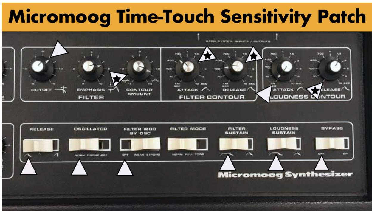
The settings shown above with a black star are *critical*, and *times* (necessarily using a *negative* CONTOUR AMOUNT) must be set depending on the speed of notes you want to play on the keyboard—facilitated by your understanding of this idea.
