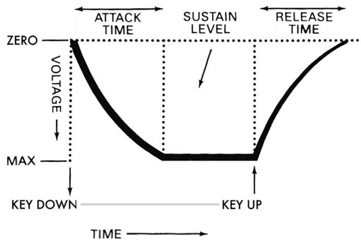
On KEY DOWN, the long ATTACK TIME in the normal Filter Contour now becomes a long (implied) "Decay Time-D" in the Inverted version! The filter starts at its highest-brightest point—the "attack" actually heard is instantaneous and bright.
